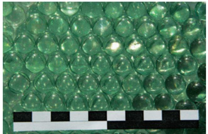
III 3b Silicate glass beads with smooth surface in the densest filling.
