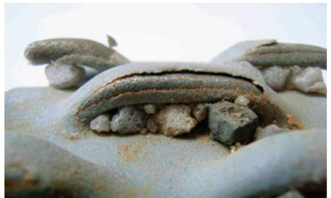
III 2 Parts of a slot bridge filter with trapped pieces of gravel and splintered quartz grains in the openings.
