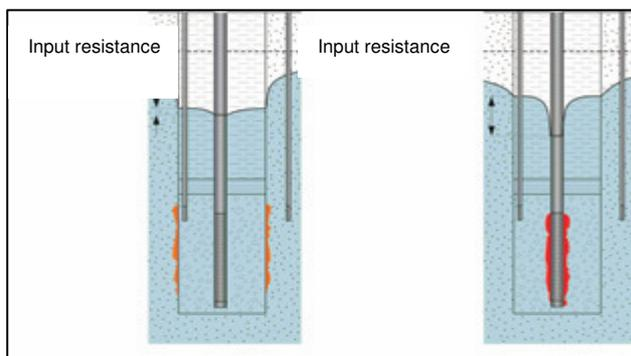
III. 1 Schematic drawing of the location of an outer (a) and inner colmatation (b) on the well.
