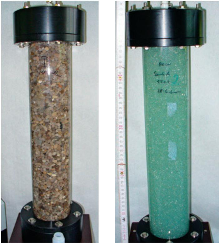
III. 4a+b Experimental pillars with filter gravel and glass beads before the start of the experiment
