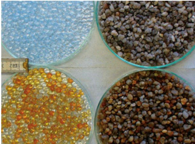
III. 7 Optical comparison of the initial material and the partially incusted material at the end of the experiment after samples were taken
