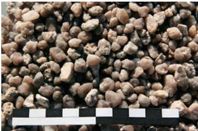
III 3a Filter gravel with irregularly formed grains and with Iron and layer silicate deposits in the cavities of the grain surfaces.
