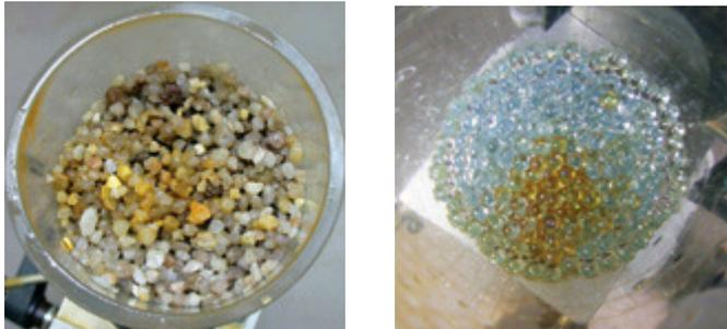
III. 5a-b Open experimental pillars with filter gravel (left) and glass beads (right) after the end of the experiment
