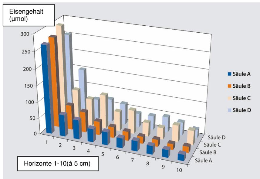
Ill. 6 Distribution of the iron masses in the 10 sampling horizons of the experimental pillars (Horizon 1 is on the inlet, horizon 10 on the outlet of the iron percolation solution)
