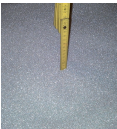
Fig. 6: 80 mm support layer, glass beads 0.75 – 1.0 mm; photo credit: ETC, Burgau
